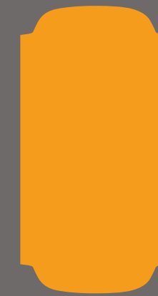
Smooth Crown Full crowned steer tire for easier turning.
